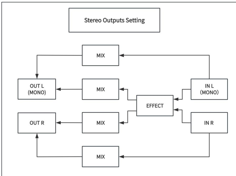
For the IN L&R, the dry (direct) and wet (delay) sounds are mixed when OUT L&R.
